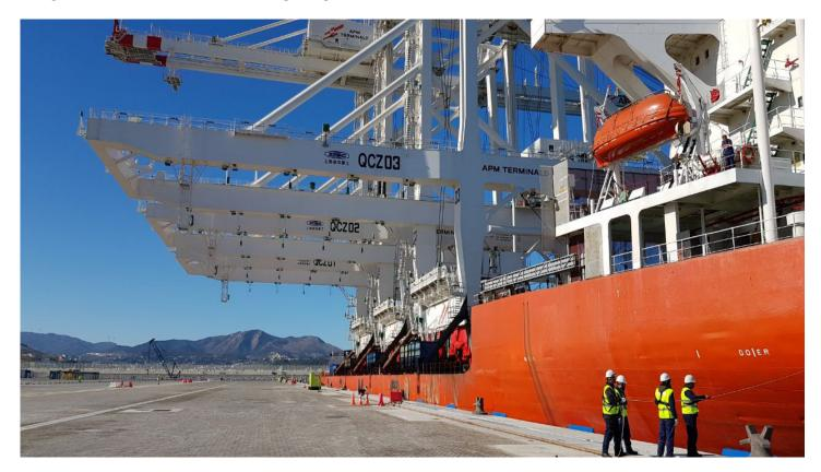
APM Terminals Med port Tangier has received its first three STS gantries, the largest in the world, designed to handle new container ships crossing the Asia / Europe trade route with capacities reaching up to 22,000 TEUs. The new Tanger Med 2 port's terminal is scheduled to be operational in 2019.
